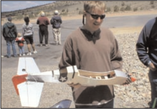
Ron Marston showing his electric Lazy P-51. Specs: wing area 750in 2 , 83 oz RTF on 12 CP2400s, Aveox 1015-1.5Y, 4.4 - 1 gearbox, 14/7 apc e-prop.
