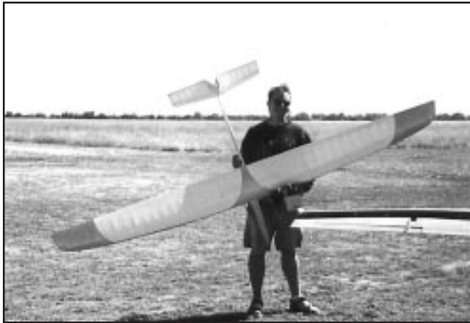
Ron Marston with his freshly rebuilt 120" RES ship. 75 oz. and about 1200 sq. in.
