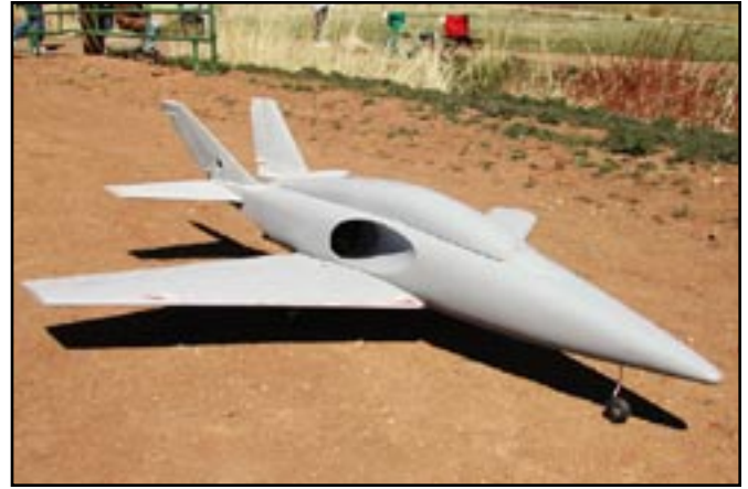
Gordon's scratch built Jet with dual brushless motors spinning a ducted fan.
