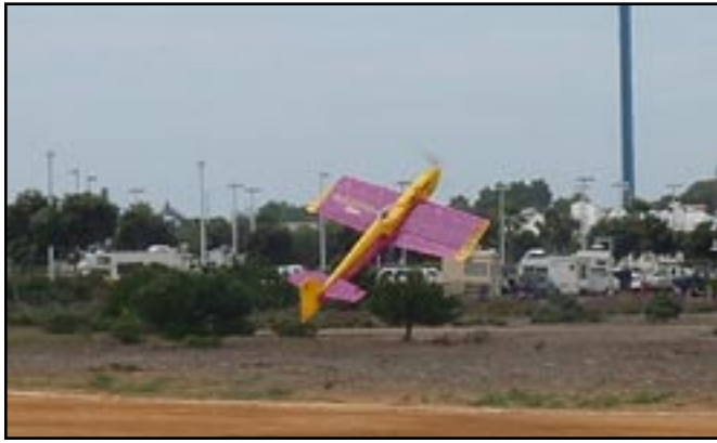
Large Diablotin powered by a large geared Hacker motor running on the new lithium-polymer batteries. Capable of 25 min full aerobatic flight.
