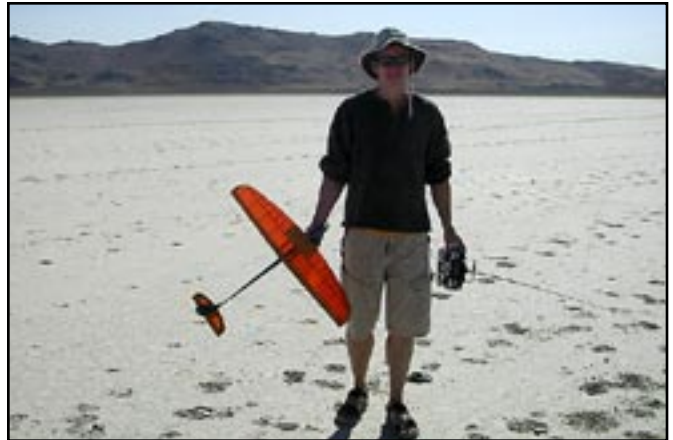
Ron Marston with his 010 Snitch at the Cold Springs dry lake. Newest version weighs 9.2 oz. RTF with a 1200 mah 3 cell Lithium battery.
