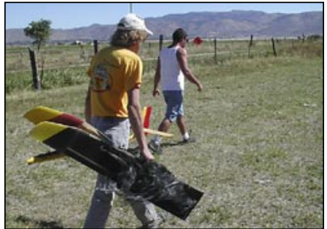
A disgusted Adam Kremers walks away from the power lines with his electrocuted plane. Note the exploded carbon in the wing.
